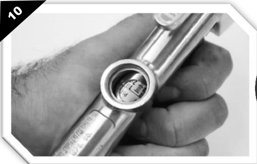
STEP #10 – Check that numbers line up within the viewing window
