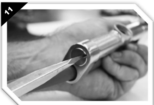
STEP #11 – Use large bladed screwdriver to tighten casting nut securely
