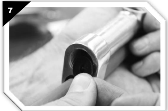
STEP #7 – NOTE – if cartridge numbers fall below viewing window, remove and add 1 or 2 additional washers until lined up correctly
